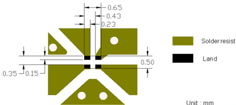
Line width should be designed to match 50Ω characteristic impedance, depending on PCB material and thickness.
