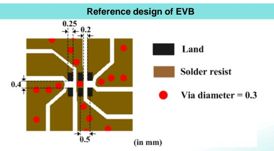
•Line width should be designed to match  $50\Omega$  characteristic impedance, depending on PCB
