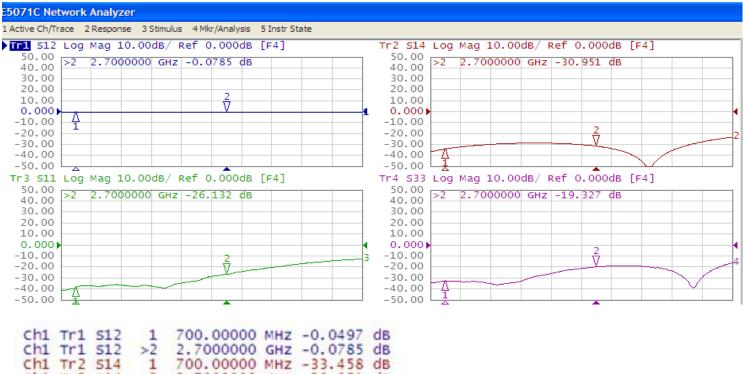
Ch1 Tr2 S12 >2 2.7000000 GHz -0.0785 dB Ch1 Tr2 S14 1 700.00000 MHz -33.458 dB Ch1 Tr2 S14 2 2.7000000 GHz -30.951 dB Ch1 Tr3 S11 1 700.00000 MHz -38.057 dB Ch1 Tr3 S11 2 2.7000000 GHz -26.132 dB Ch1 Tr4 S33 1 700.00000 MHz -32.191 dB Ch1 Tr4 S33 2 2.7000000 GHz -19.327 dB
