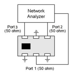
Test Instrument: Agilent E5071C Network Analyzer or equivalent.
