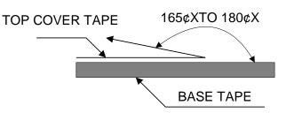
The force for peeling of cover tape is 10 grams in the arrow direction.
