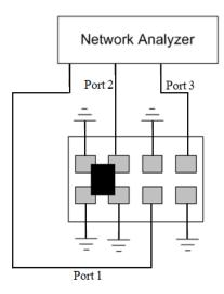
Test Instrument : Agilent E5071A Network Analyzer
