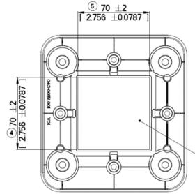
Adhere the adhesive tape in the recession of the bracket
