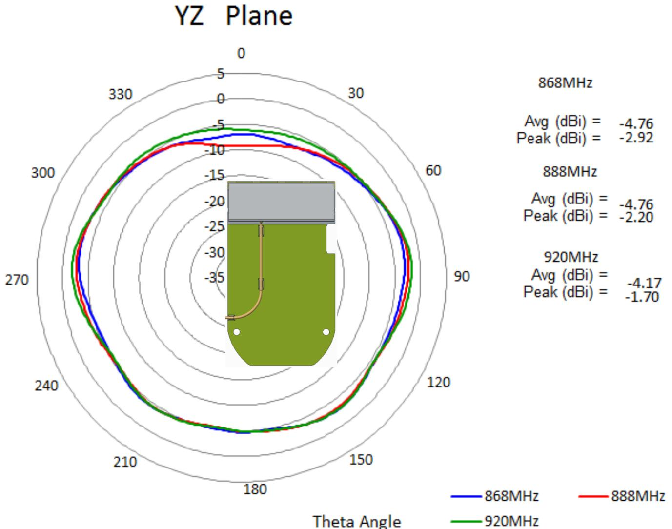
Test PCB size: 67.8mm\*39.6mm
