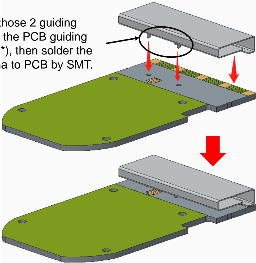
\* The 2 guiding holes on PCB must be non plated holes without any metal.
