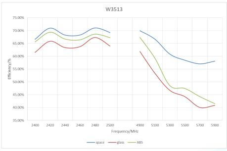
When placed on ABS or glass, mainly difference is in high frequency band(4.9G-5.9G). Which performance will decline.
