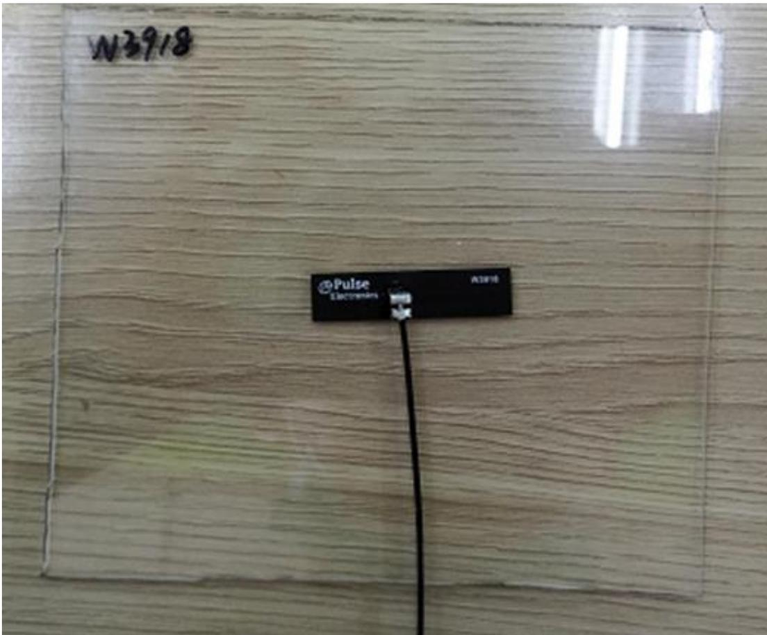
***(\*) All RF parameters measured on 2mm thick PC plate***
