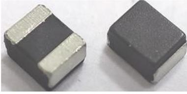
The BDCC series is the special design to enhance the performance of PFM and PWM applications. It provides lower Rac value at light load and lower Rdc value at heavy load to improve efficiency performance. Furthermore, it provides excellent saturation current to reduce the ripple current and enhance efficiency.
