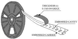
The force for peeling of cover tape is 10 grams in the arrow direction.
