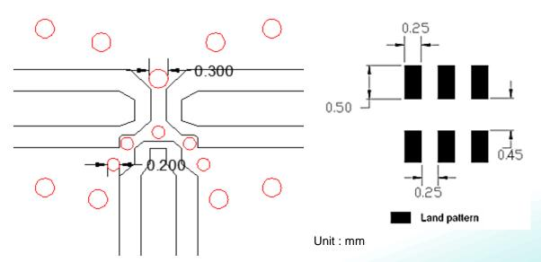
\*Line width should be designed to match 50Ω characteristic impedance, depending on PCB material and thickness.
