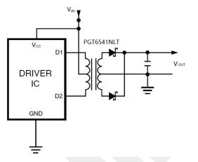
For a fixed 50% duty cycle mode of operation, the output voltage is simply determined by the input voltage and turns ratio. So, with the available turn ratios, a variety of output voltages can be met.
