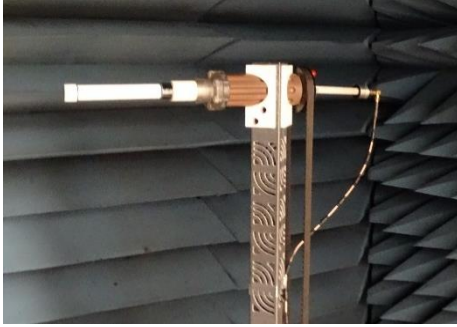
RO2471NM antenna sample measured in free space
