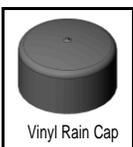
To combat this problem, all Larsen NMOHF mounts will be shipped with a disposable vinyl rain cap. The rain cap can be installed for outside vehicle storage or other sources of moisture. For vehicles with NMO mounts that may be exposed to the elements for the long term, Larsen recommends that they be stored with antenna bases attached or order the more durable NMO rain cap (part number NMOCAPB).
