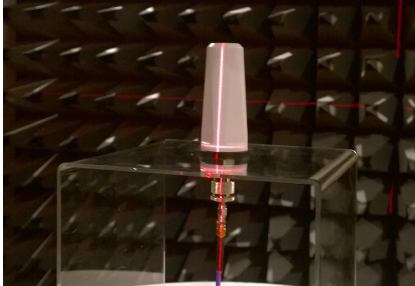
LPTNGP600/71DMN antenna sample measured without ground plane.
